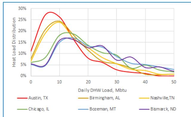
Figure 18 – Annual Water Heating Load Frequency Distribution
