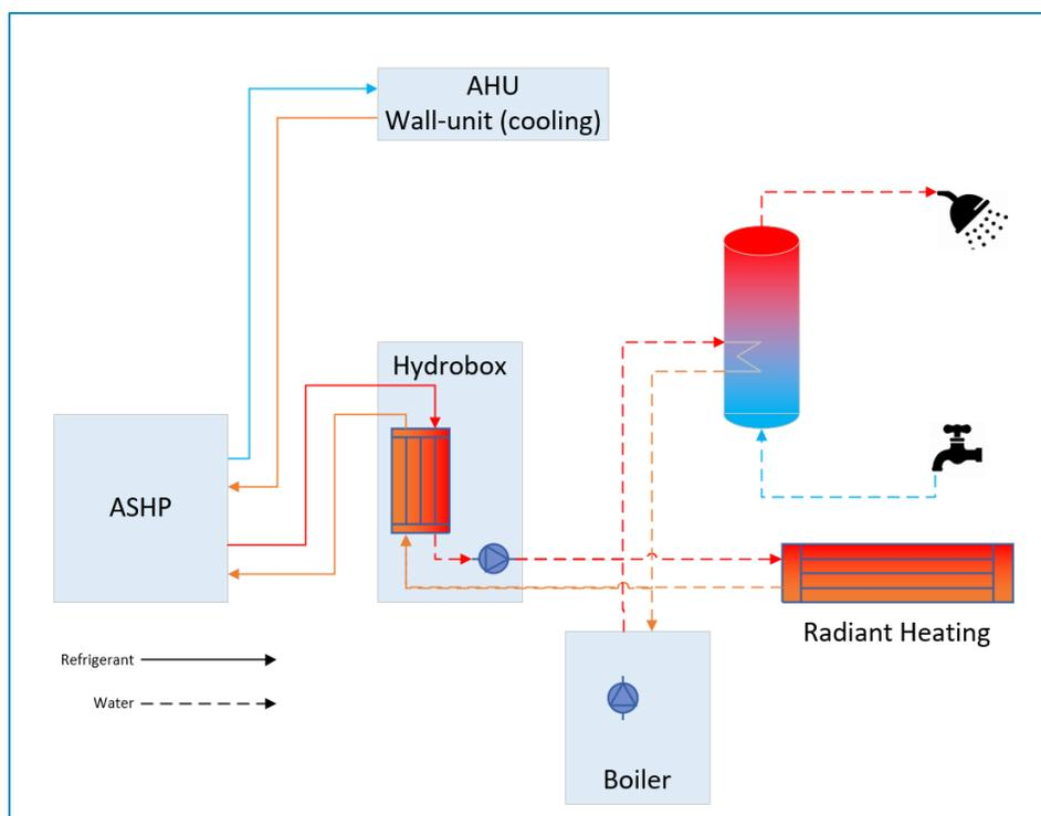
Figure 2 – Boiler Integration with A2WHP Systems
