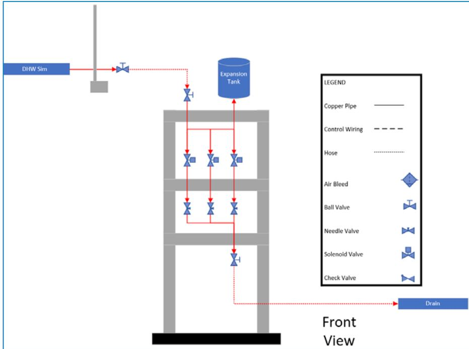
Figure 20 – Domestic Hot Water Simulator P&ID
