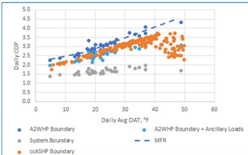
Figure 7 – A2WHP system and ccASHP COP Performance Comparison
