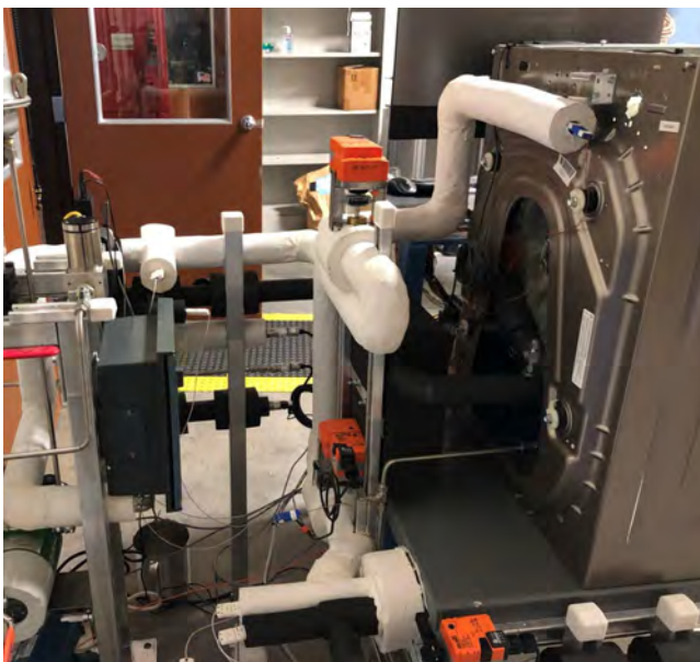
Photos illustrate the technology prototype infrastructure laboratory testing facilities. The modified commercial dryer was tested for drying performance evaluation and comparison with state-of-the-art technology.
