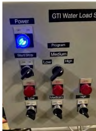
Water heater with damper, data acquisition system and water load simulator for testing (left). Programmable water load simulator (right)
