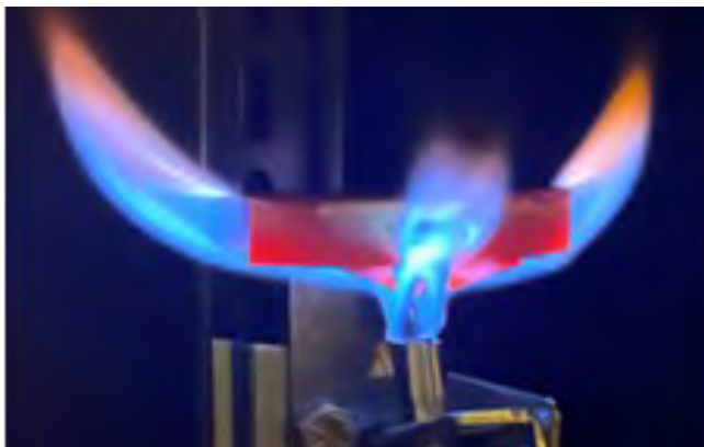
Fryer pilot light using 100% natural gas.
