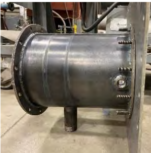
Sideview and combustion air inlet ends of the fabricated Design II burner section housing the nozzle assembly
