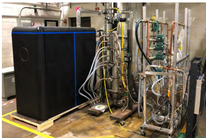
Experimental test stand with carbon capture unit (left), water-heater simulator (middle), and recirculation loop (right).
