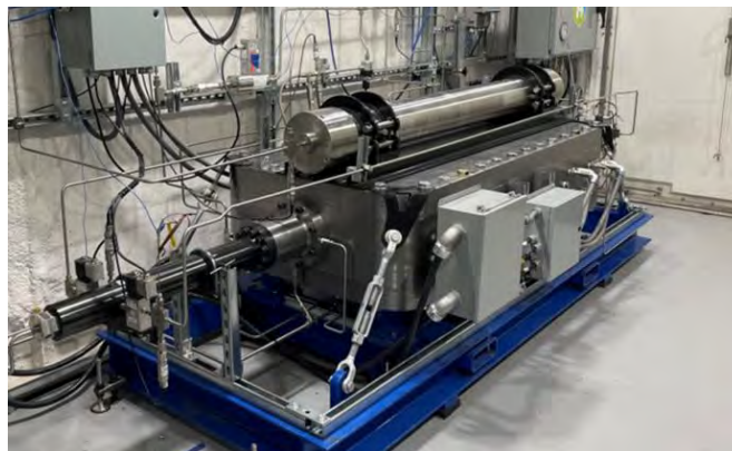
Fabricated expander currently being tested in laboratory.
