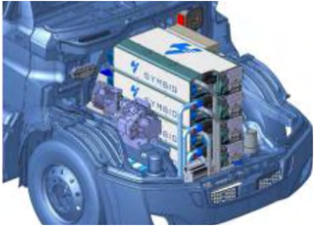
Proposed envelope for fuel cell and low temperature thermal management equipment
