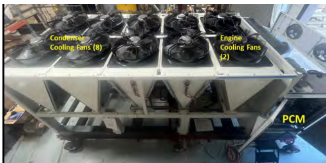
Hybrid chiller prototype construction cell
